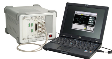
U2761A used as a modular instrument
