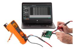
Utilize the U5404A remote switch probe to measure, save and send measurement readings over to Keysight handheld meter logger software with just a press of the button.
