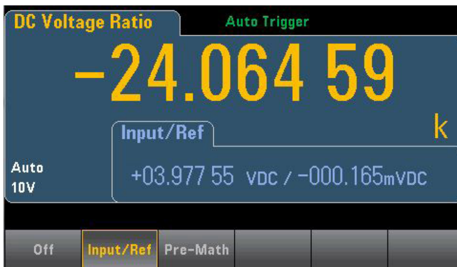
Figure 6. Here, the Input/Ref measurements are displayed independent of the ratio measurement.
