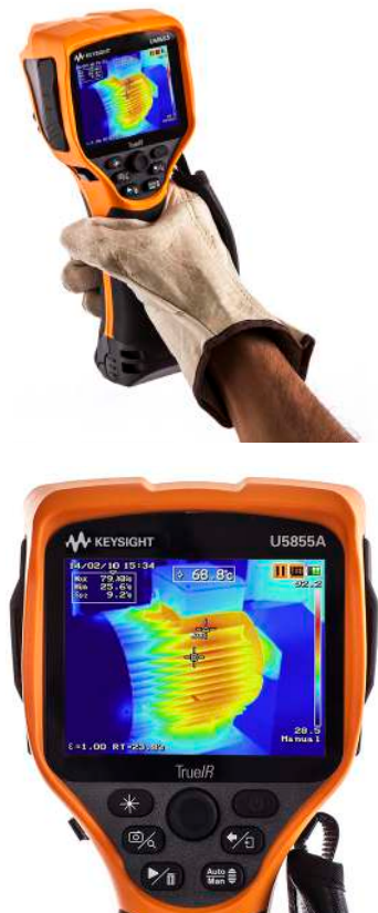
Figure 2. U5855A TrueIR thermal imager
