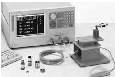
4287A RF LCR meter 1 MHz to 3 GHz
