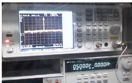
Figure 4 Testing system – N9320B RF spectrum analyzer, E3632A power supply and 34401A digital multimeter
