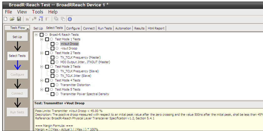
Figure 2. The Keysight automated test engine quickly guides you through selecting and configuring tests, setting up the connection, running tests, and viewing results. You can easily select individual tests or groups of tests with a mouse-click.
