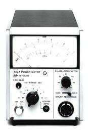
As today's power measurements become more complex, it is increasingly difficult to make reliable, accurate power measurements. For more than 40 years, you've depended on Keysight's 432A analog power meter, used with temperature compensated thermistor sensors to provide high accuracy over a wide temperature range.
