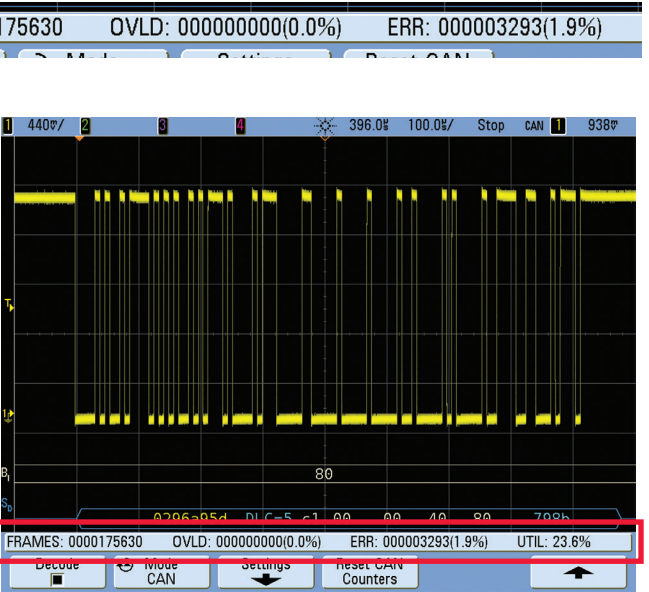
Figure 2. Real-time totalize functions provide CAN bus efficiency and quality measurement statistics.
