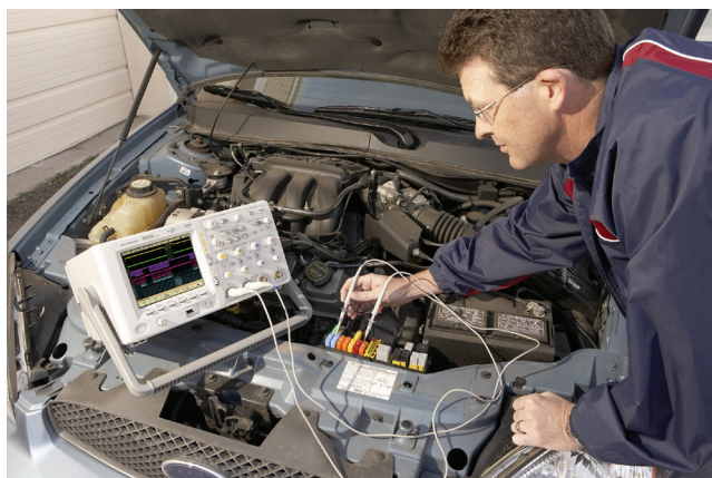
Figure 9. Making remote CAN and LIN measurements with Keysight's battery option for InfiniiVision Series scopes.
