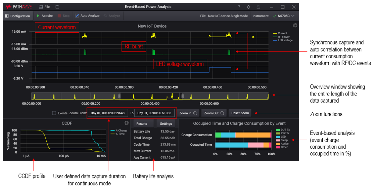
Figure 4. Overview of the KS833A2A event-based power analysis software
