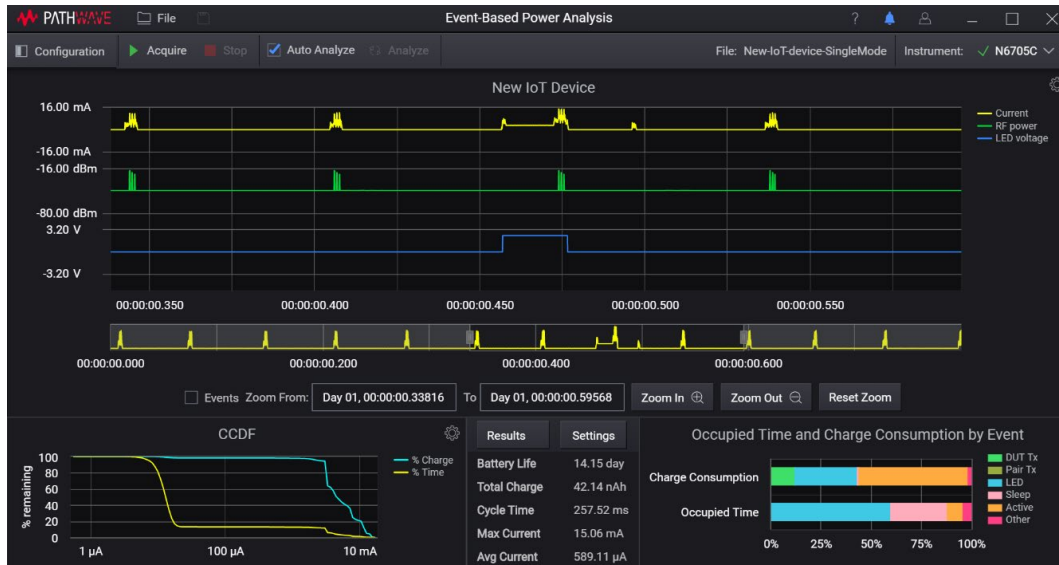
Figure 13. Battery life predicted based on four full operational cycles and 0.2-Ah battery capacity
