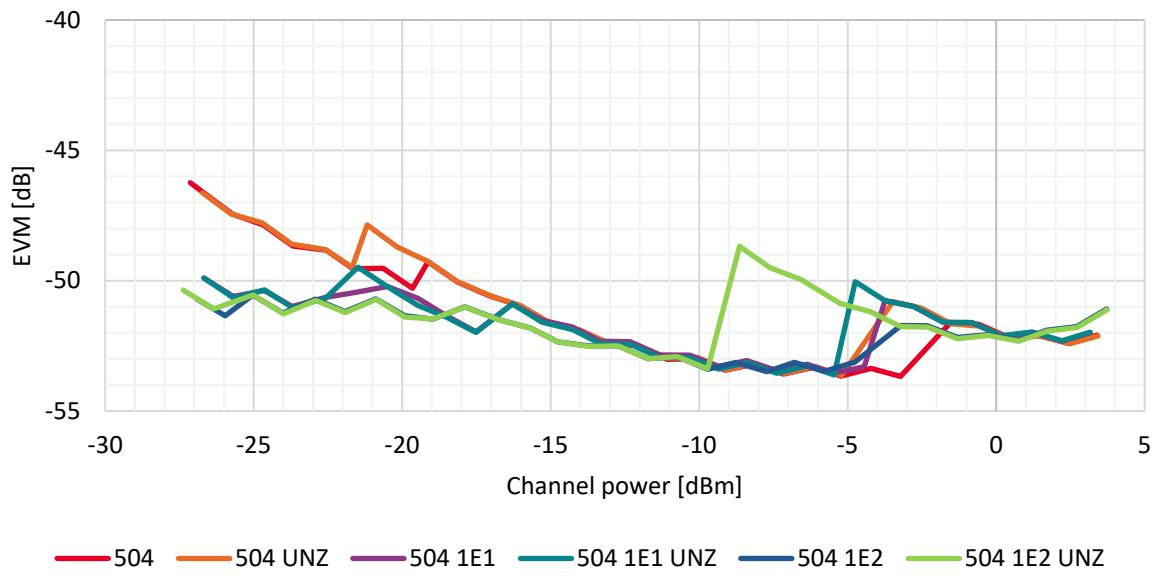
Measured EVM vs. power vs. options at 3 GHz
