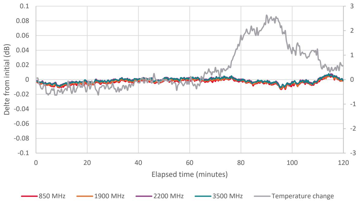
Repeatability measures the ability of the instrument to return a given power setting after a random excursion to any other frequency and power setting.
