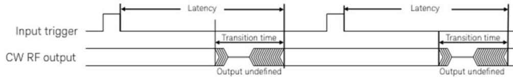
Latency and RF transition time for frequency changes (F1-F3) and amplitude changes (A1, A2) (measured)<sup>2</sup>
