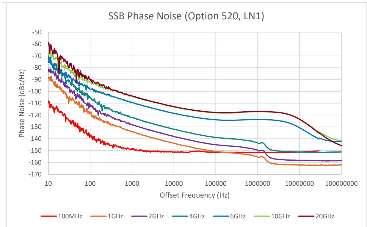
Absolute SSB phase noise (CW) at +10 dBm or maximum output power in dBc/Hz, (measured) (Option LN1 + UNZ), [ ] = Option LN2 + UNZ
