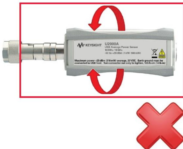
Figure 6. Do not turn the power sensor body
