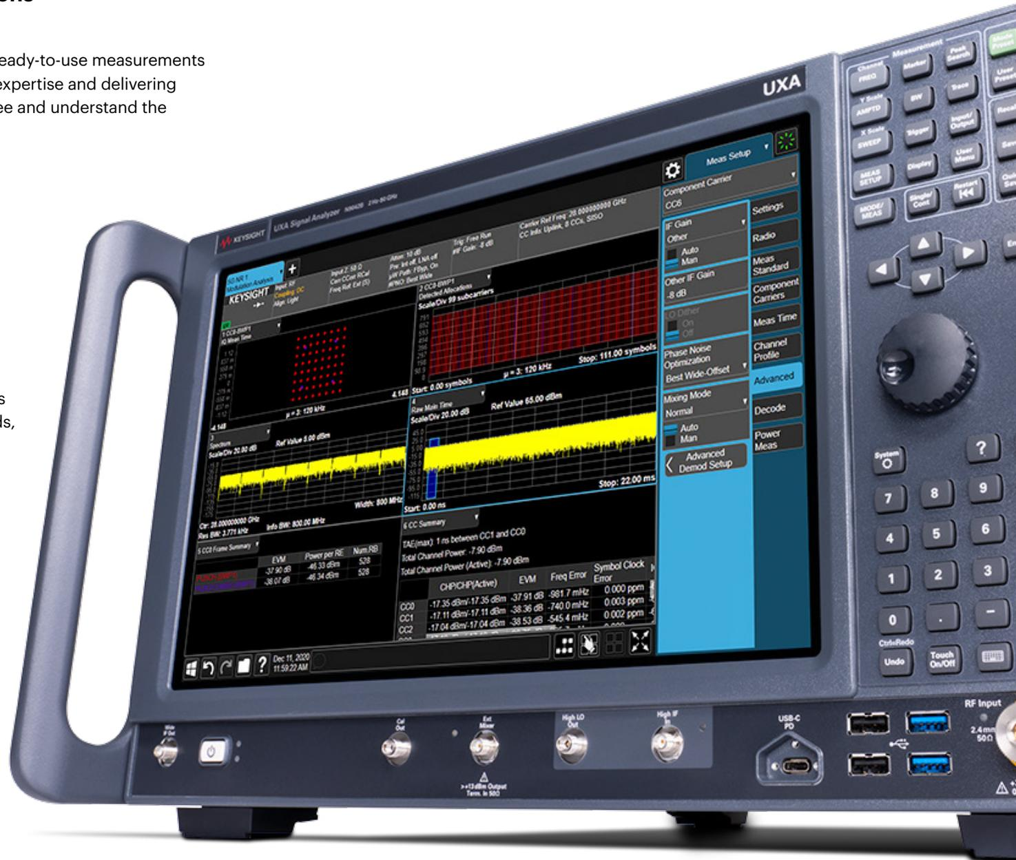
N9042B UX A X-Series Signal Analyzer
