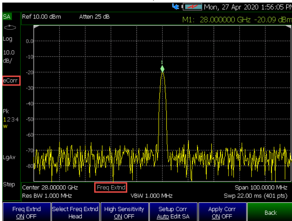
Figure 30-5 FieldFox Frequency Converter (Freq Extend) On And Corrections (eCorr) Enabled (SA mode shown; other compatible modes are similar.)
