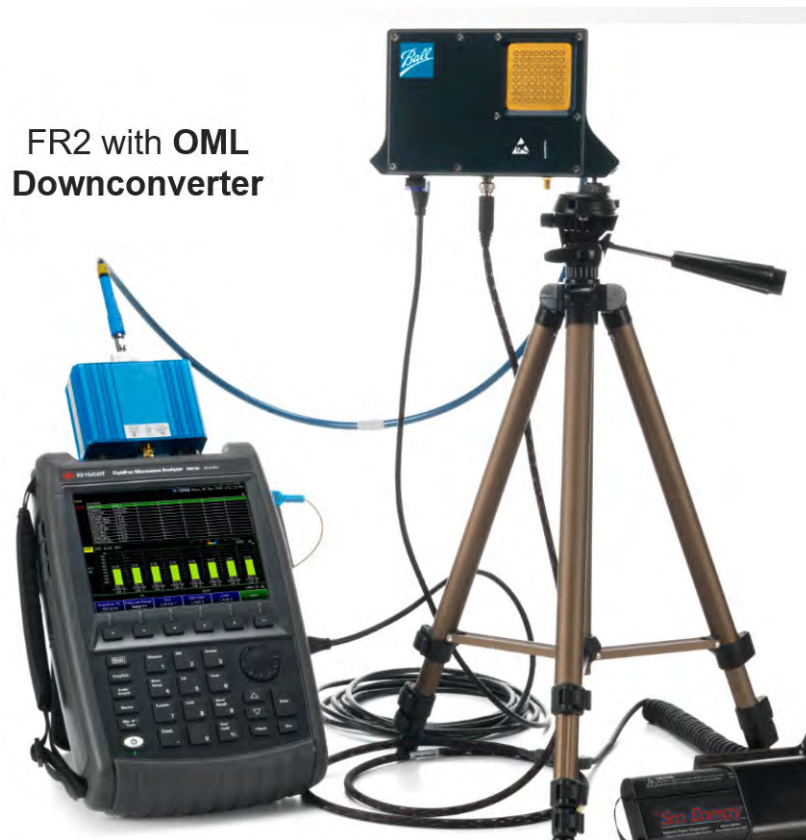
Figure 30-1 FieldFox with OML Downconverter
