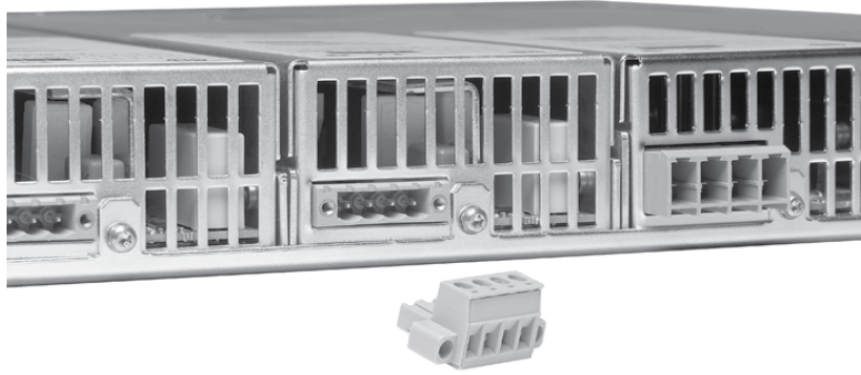
Figure 5. Quick disconnects for power and sense leads
