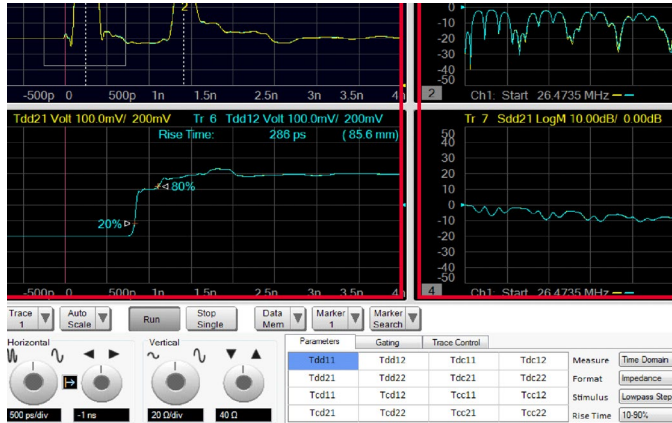
Figure 25. Measurements are taken as a function of frequency. The frequency domain information is used to calculate the Inverse Fourier Transform for time domain results.
