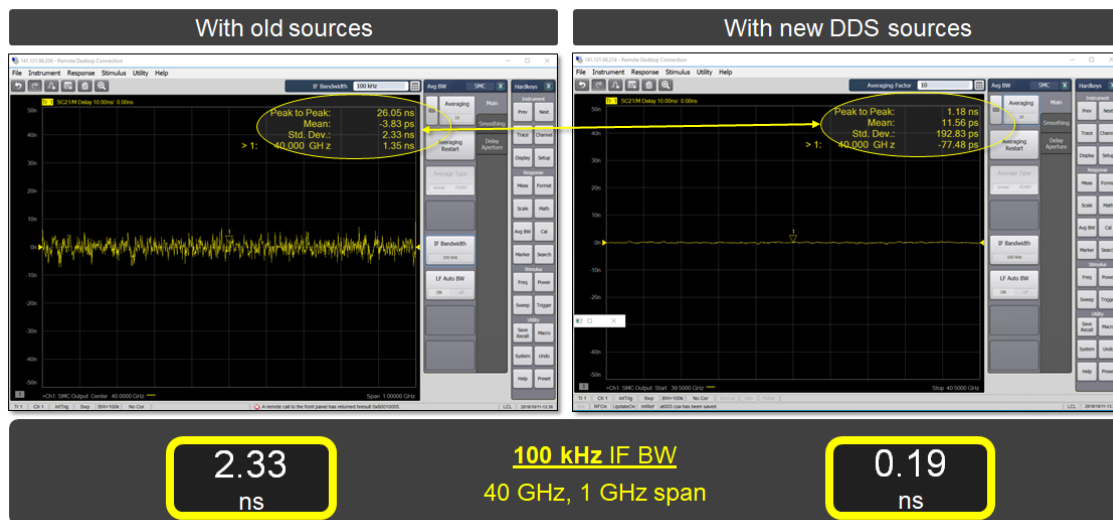
Mixer group delay measurement with SMC+phase application
