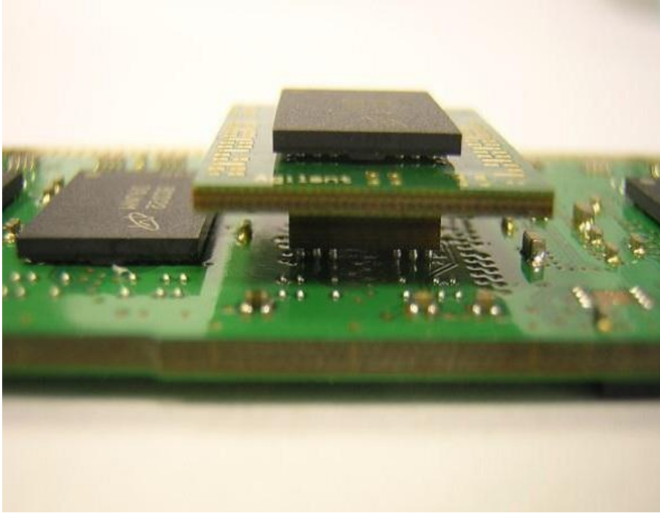
Figure 1. Photo of stacked DIMM-Riser-Interposer-DDR.
