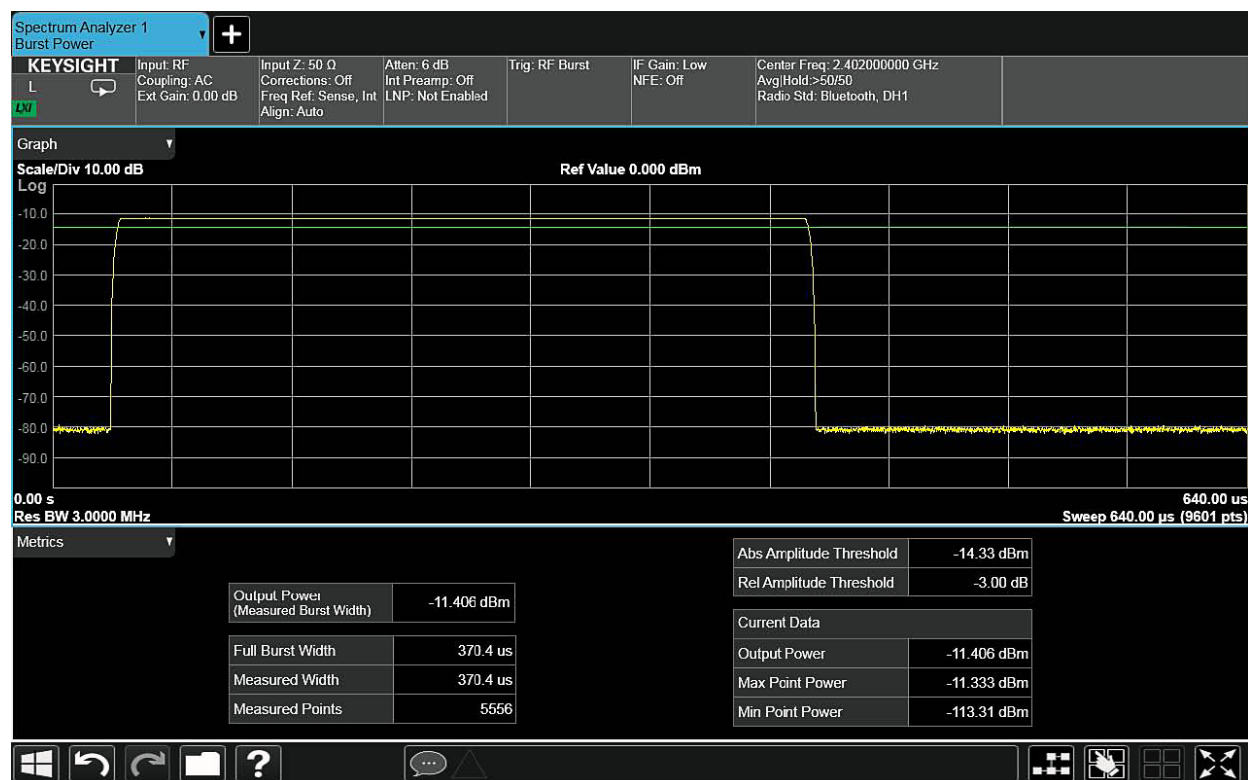
Figure 5. The table below the measurement trace provides a summary of key metrics for the power of a burst signal.
