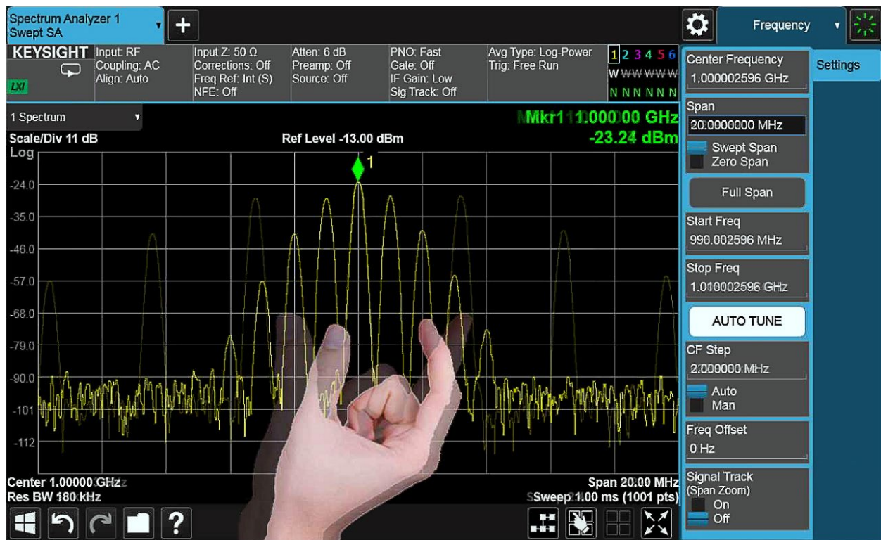
Figure 7. Changing the vertical or horizontal resolution of the display is as easy as touching the screen and spreading or pinching two fingers.
