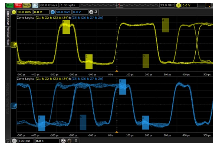
Figure 2. The standard InfiniiScan software enables you to isolate a signal anomaly with ease.
