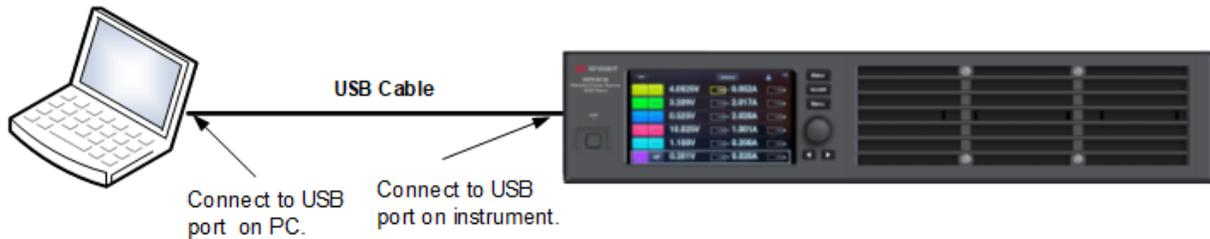
1. Connect your instrument to the USB port on your computer. Note that a USB-C interface cable is required, preferably one with a locking connector.
