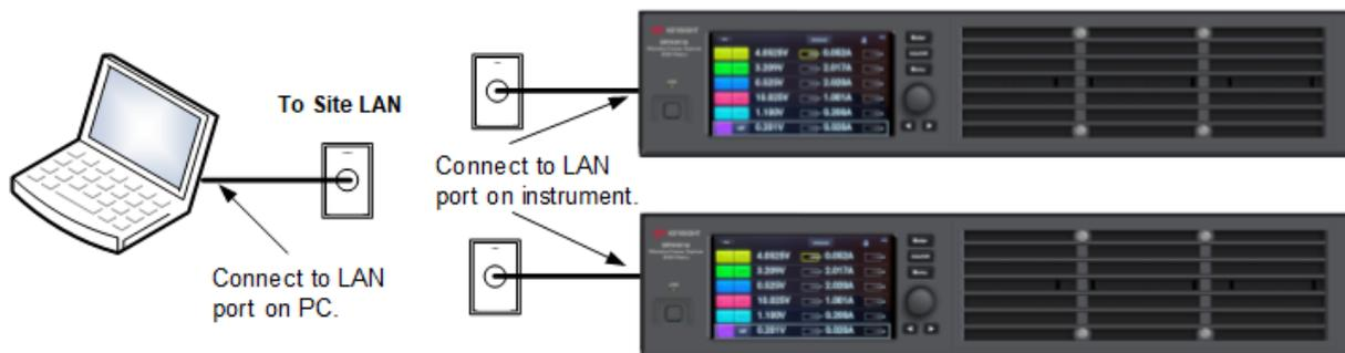
A private LAN is a network in which LAN-enabled instruments and computers are directly connected, and not connected to a site LAN. They are typically small, with no centrally-managed resources. The following figure illustrates a typical private LAN system.
