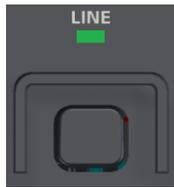
The **Line** switch turns the unit on or off. The green LED indicates power is on.
