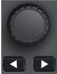
Use the rotary knob (RPG) to navigate around the display. Push on the knob to select an item. When a numeric field is selected, the touch screen numeric keypad will pop up. When a text field is selected, the list will pop up; rotating the knob scrolls through the options. Pushing the knob again will choose the option from the list.
