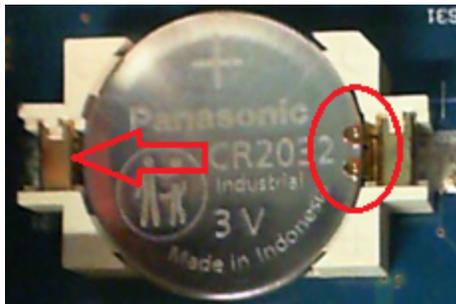
3. Install the new battery. Make sure that the positive side (+) is facing up. Place the battery *under* the small spring clips indicated by the circle, then push down on the opposite end of the battery indicated by the red arrow. The top of the small spring clips should be visible after the battery is seated (see red circle)
