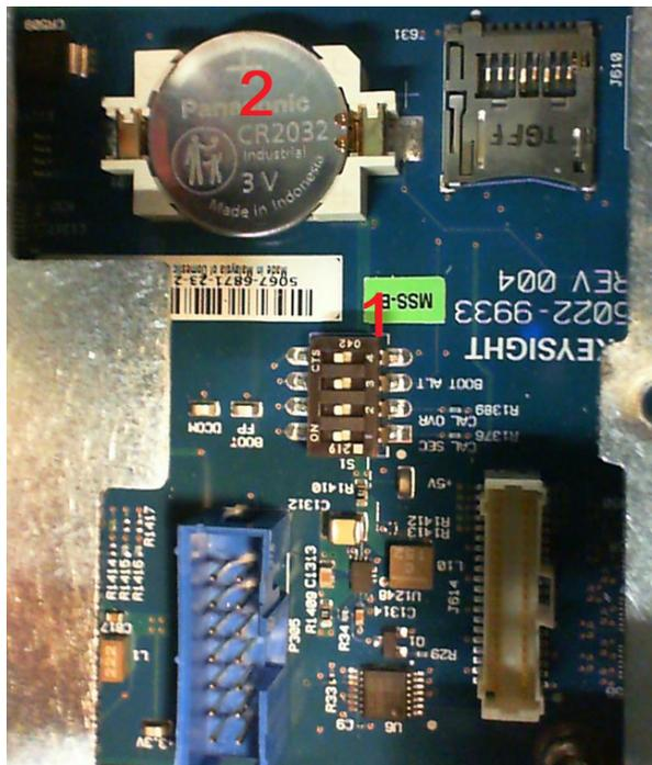
4. When calibration switch settings or battery replacement is complete, reinstall the shield if you do not have a GPIB card.
