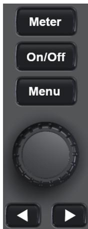
The **Meter** key returns the display to metering mode. It also toggles between All Channel view and Single Channel view.
