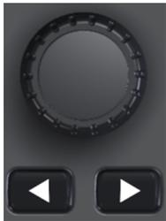
Use the rotary knob (RPG) to navigate around the display. Push on the knob to select an item. When a numeric field is selected, the touch screen numeric keypad will pop up. When a text field is selected, the list will pop up; rotating the knob scrolls through the options. Pushing the knob again will choose the option from the list.
