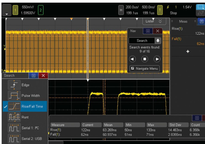
Figure 10a. The 4000 X-Series was set up to capture data signals with various rise time edges. Using the search and navigation capability, the oscilloscope was able to find, mark (white triangles), and quickly navigate to 16 occurrences of “out of compliance” rise-time
