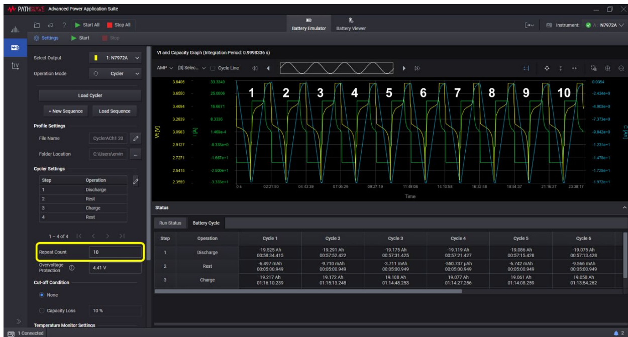
Figure 14. Cycler with battery voltage, current, and capacity graph (top), and a cycle capacity table (bottom).
