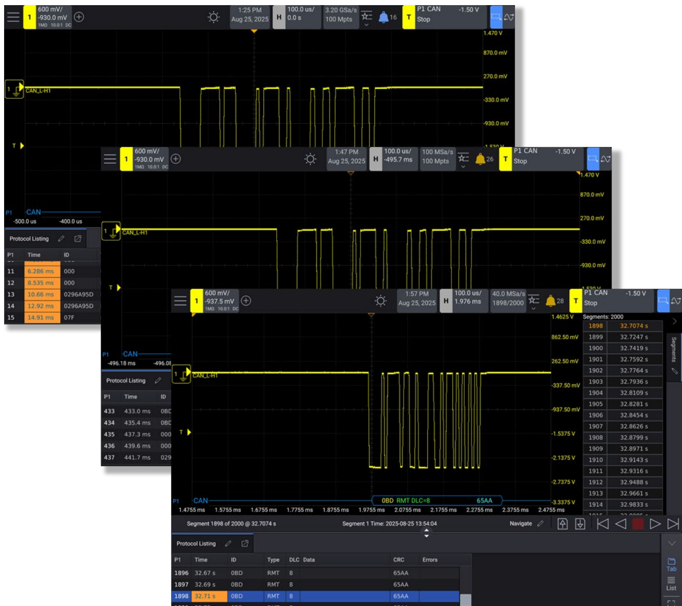
Controlling sample rate with CAN protocol decode
