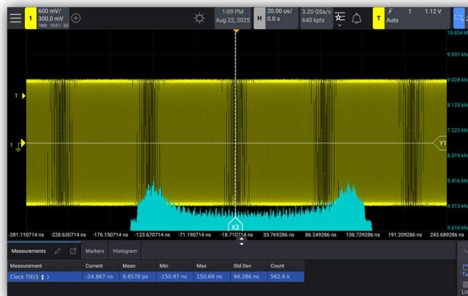
Clock TIE measurement using the HD300QJTA software application
