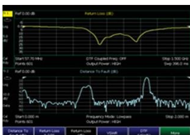
View return loss and DTF simultaneously
