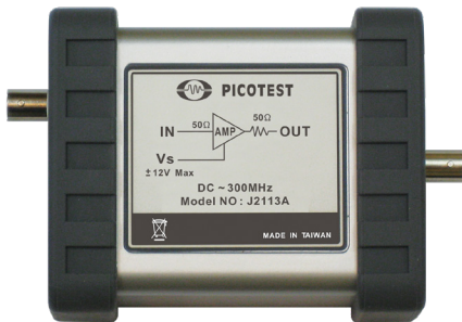
Picotest J2113A Semi-Floating Differential Amplifier
