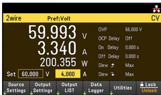
Figure 2 a. The E36231A and E36232A can display many more details simultaneously, including the present output, measured output, OVP/OCP condition, and delays.
