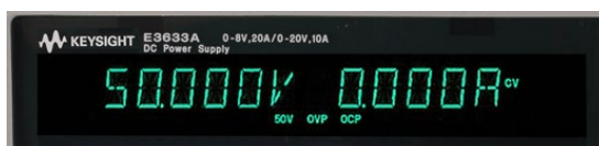
Figure 2 b. The E3633A and E3634A only display one channel setting (current and voltage) at a time.
