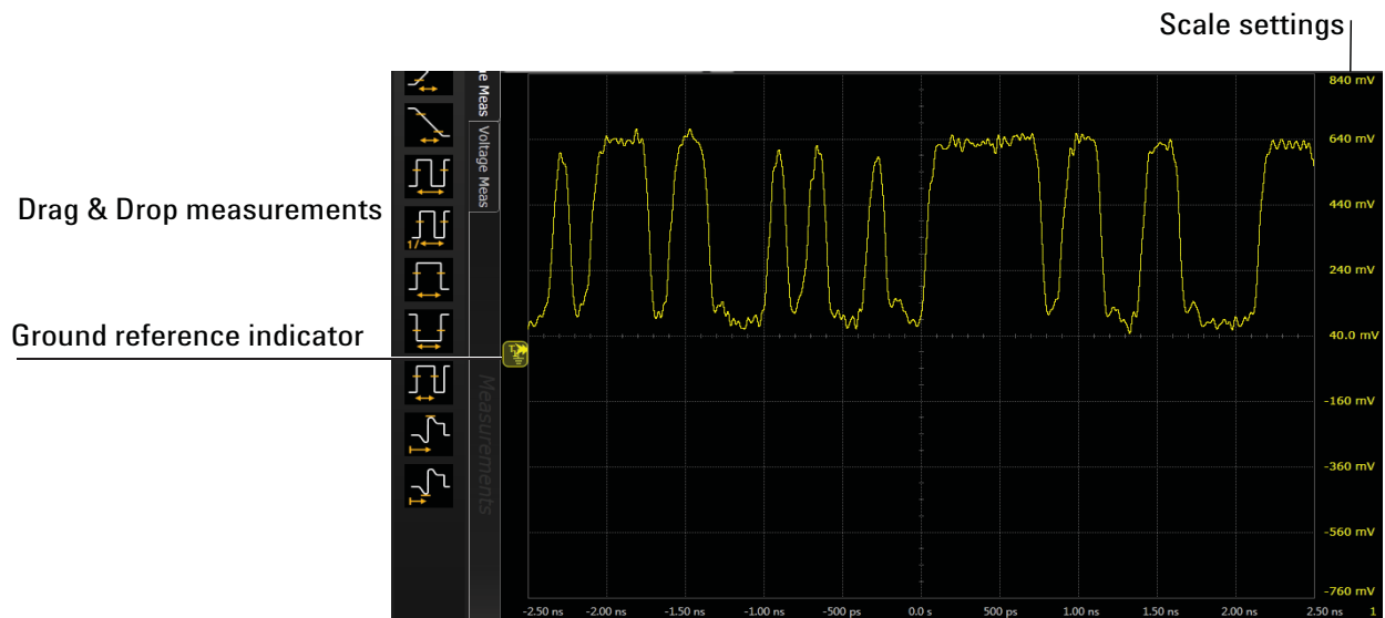
Figure 9 Infiniium oscilloscope waveform display area
