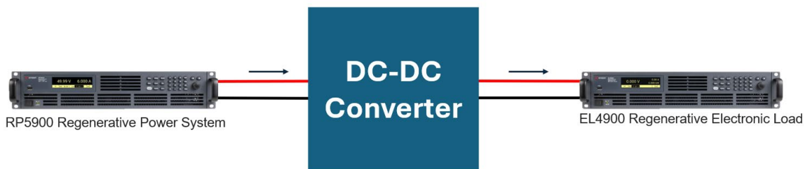
Figure 10. DC-DC converter efficiency test setup with Keysight RP5900 and EL4900
