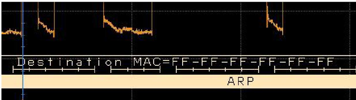
Figure 8. Protocol decode in waveform area
