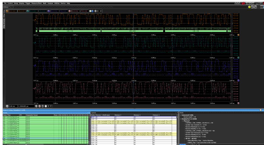
Figure 9. DisplayPort 2.1 UHBR trigger and decode, with protocol lister and detailed packet view.
