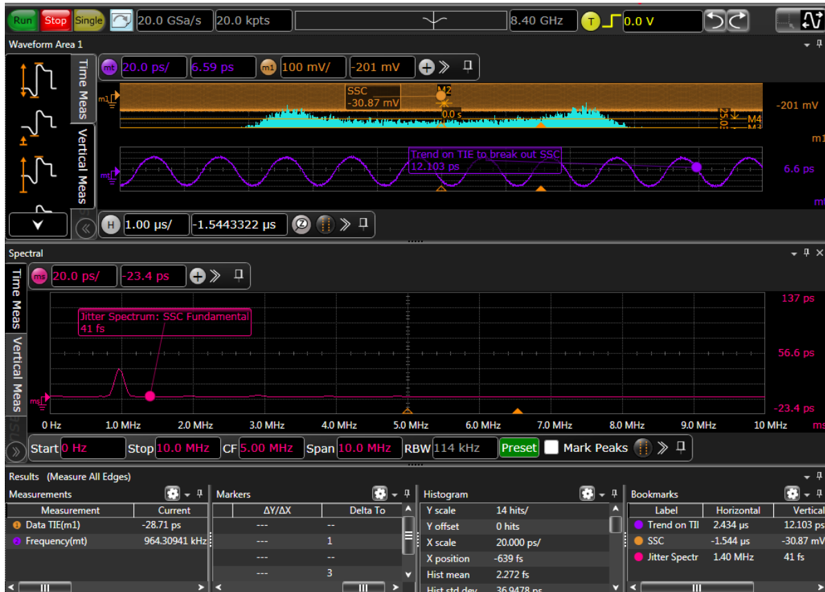
Figure 5. Results of the measurement setup wizard show the jitter histogram, trend, and spectrum.
