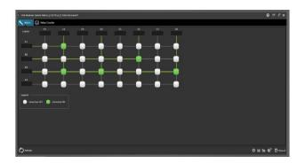
Easily open and close relays channels on your USB Modular switch matrix.
