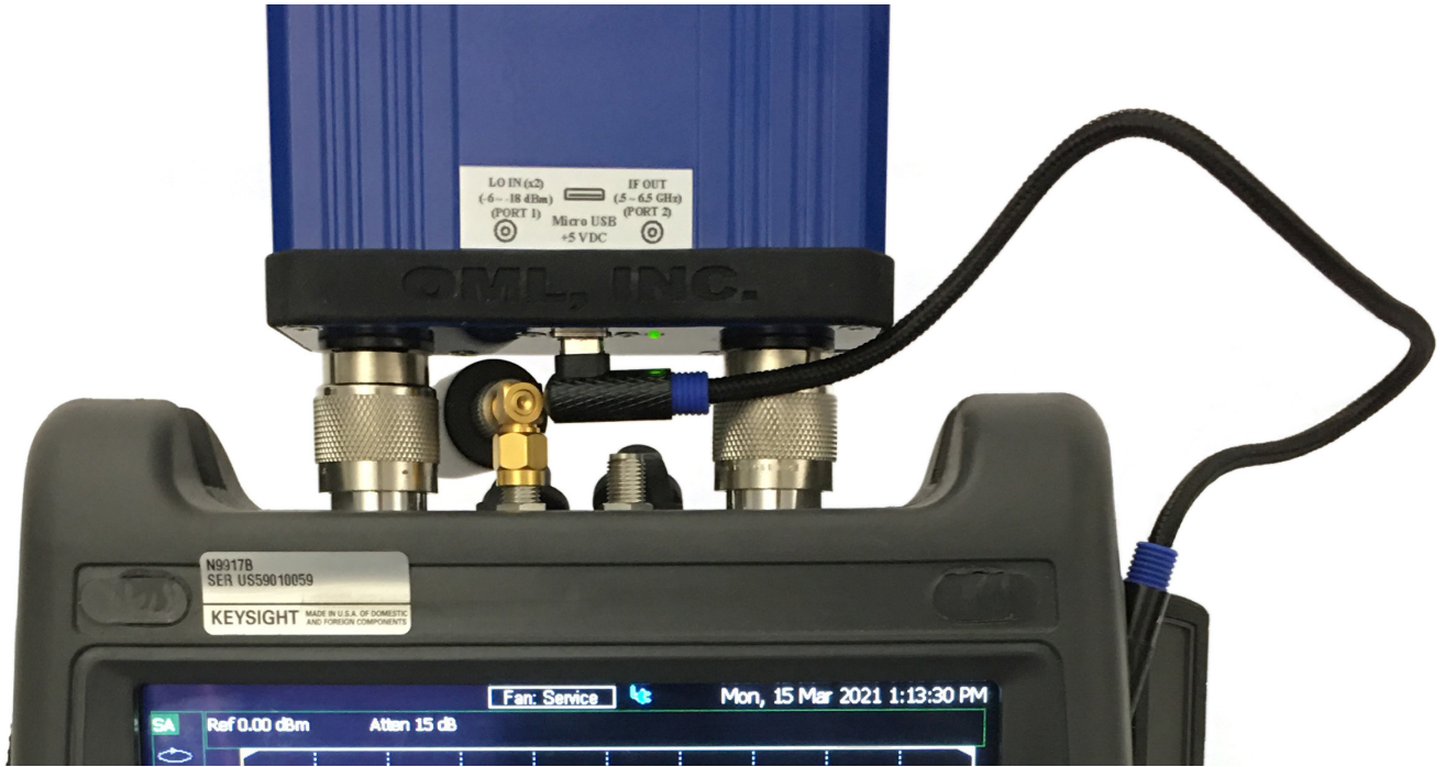
Figure 4 Example of model N9910XM28-H2N connected directly to a N9917B 18 GHz FieldFox. Note that the Ref/Trig input connector is blocked by the mini USB connector.
