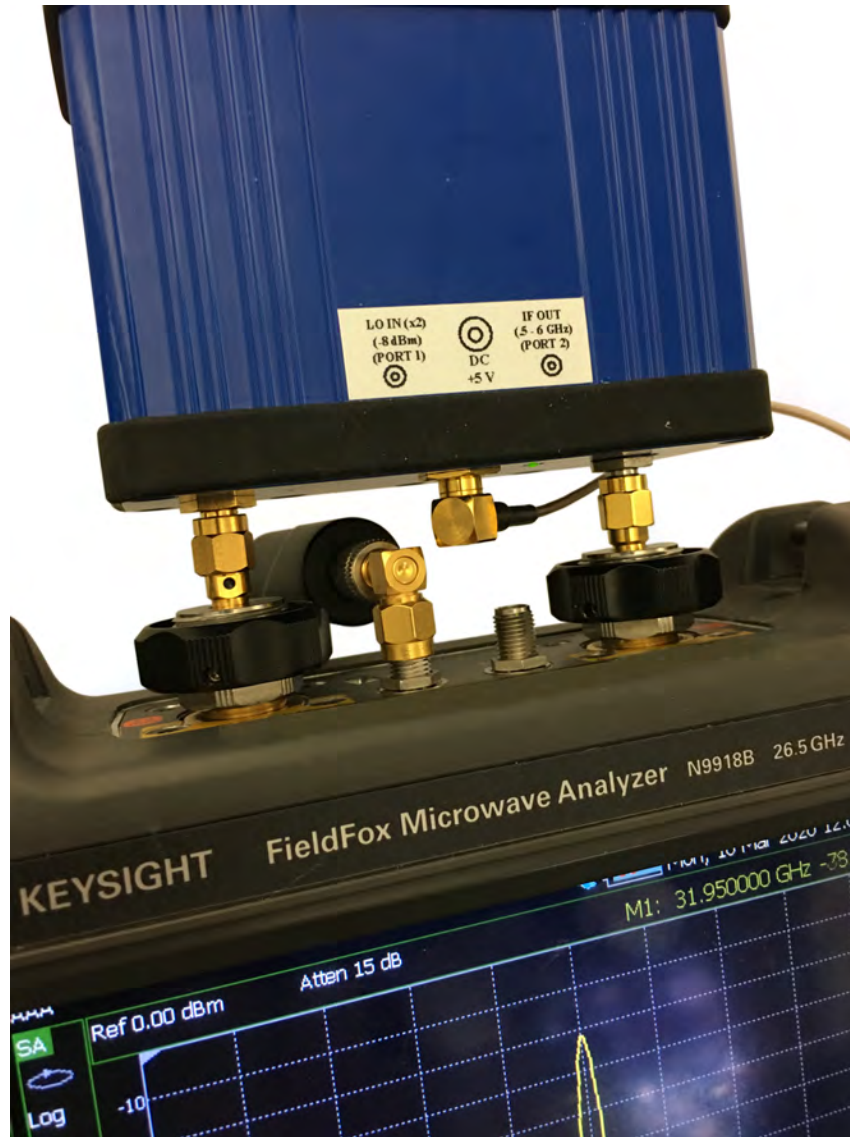
Figure 3 Example of Adapter Kit N9910XM28-AK3 for connecting FieldFox analyzers with 3.5mm Port connectors directly to the mixer. N9910XM28-AK4 is used to attach the GPS antenna at a right angle.
