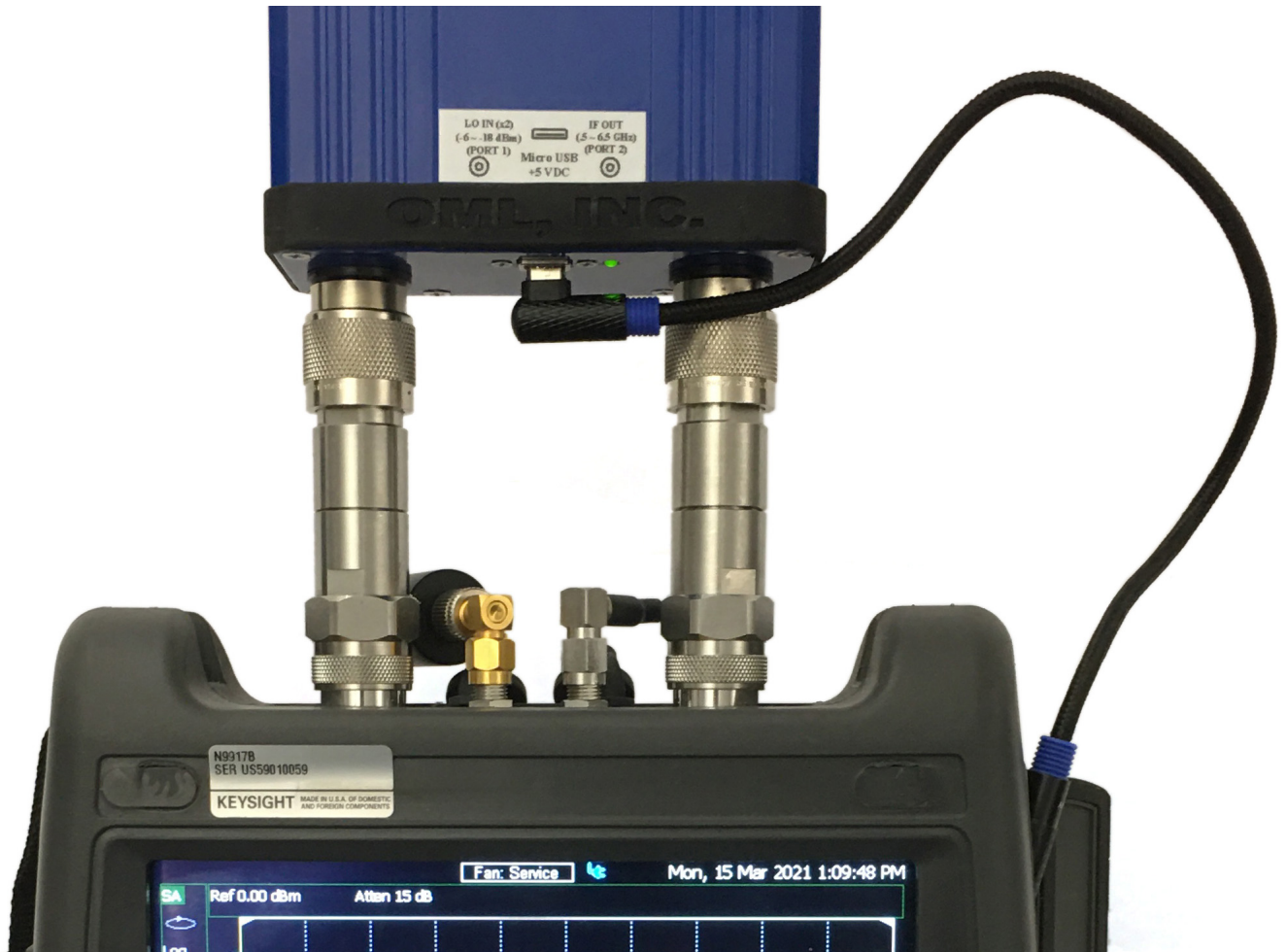
Figure 5 Example of the N9910XM28-H2N Mixer connected with Adapter Kit N9910XM28-AK6. The -AK6 acts as a spacer to allow access to the Ref/Trig connector.
