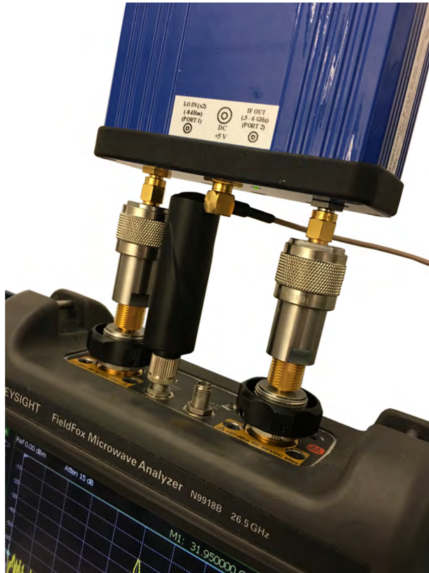
Figure 2 Example of Adapter Kit N9910XM28-AK1 and N9910XM28-AK2 connected together to act as a spacer for the vertically mounted GPS Antenna. This is for FieldFox analyzers with 3.5 mm Port connectors.
