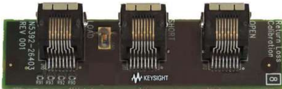
Figure 8. The return loss fixture is used to calibrate the VNA for return loss measurements and is included in the standard Ethernet fixture kit.
