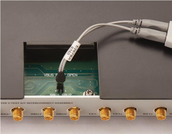
Figure 6. Use the E2678B socketed head with InfiniiMax I/II probe amp to probe D+/D- signals.
