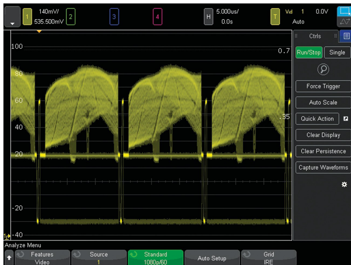
Figure 27. Triggering on 1080p HDTV signal analysis.
