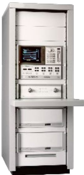
Figure 1. By the 1990s, the HP 8510 was the industry-standard for pulsed-RF vector network analyzers
