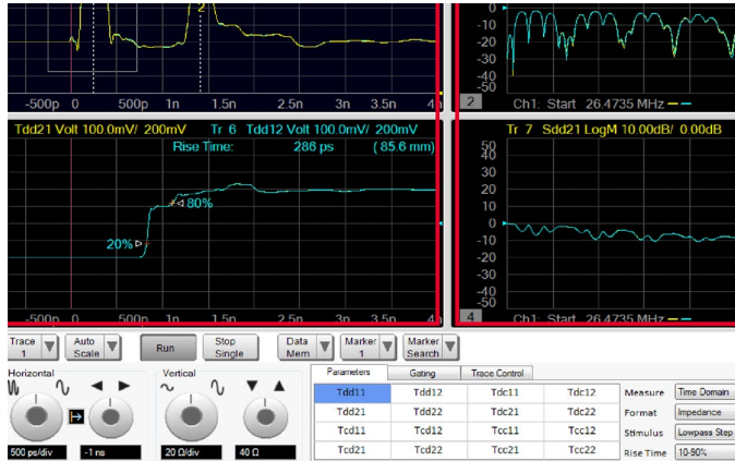
Figure 27. Measurements are taken as a function of frequency. The frequency domain information is used to calculate the Inverse Fourier Transform for time domain results.
