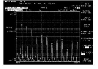
Harmonic markers are used to calculate the THD of a signal without including the effects of noise.
