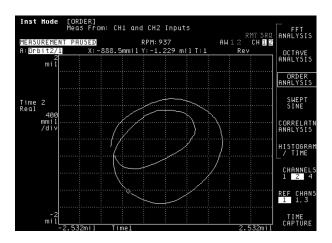
Oscilloscope-quality orbit diagrams mean you carry only one instrument onto the shop floor.
