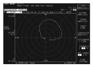
Markers are used to annotate shaft speeds at selected points in a run-up measurement.
