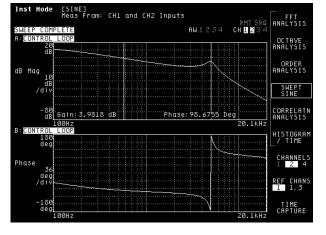
The stability of a control loop is quickly characterized using the gain and phase margin marker function.
