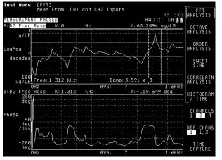
Characteristics of a selected resonance are automatically calculated from an impact measurement using the frequency and damping marker.
