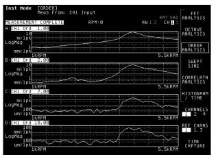
Order tracking is used to simultaneously display up to four orders or a combination of orders, composite power and RPM profile.
