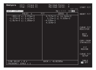
Curve fit provides an exact mathematical model of your circuit or device.
