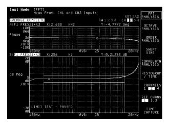
Limits are used for go/no go testing in production. The response of an accelerometer is being checked in this example.
