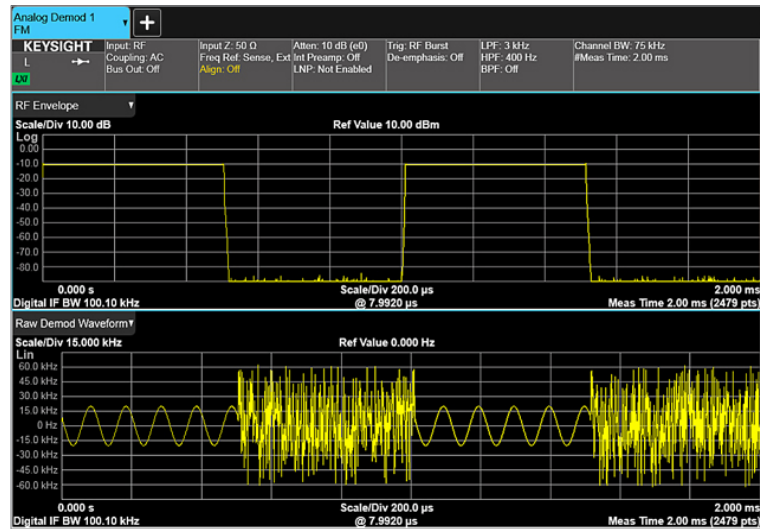
Figure 6. "Transient Analysis" view helps quantify the transient events in time domain.
