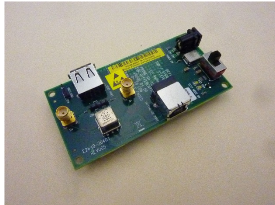
Figure 7. E2666B hi-speed device test fixture.
