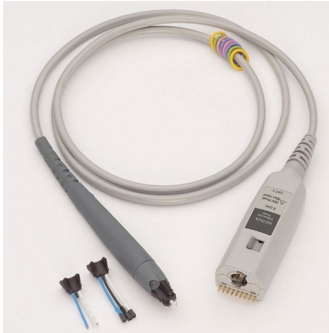
Figure 13. Keysight's InfiniiMode N2750A Series differential active probe.
