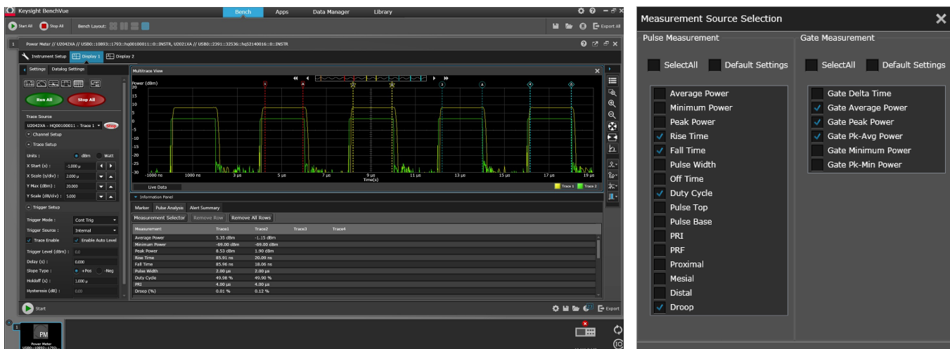
Figure 11. Multi-channel trace display with 4-pairs of gates and automatic pulse parameters measurement (sample screen shot with two X-Series power sensors).
