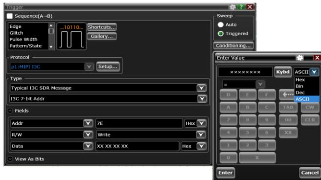
Figure Using up to 3 field values of specific packet type, it is possible to trigger on specific pattern that you want to see.
