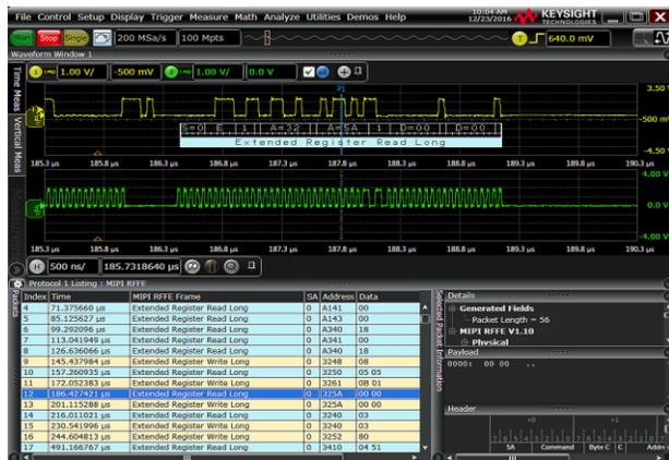
Figure A dual view showing the physical layer with a time-aligned decode, as well as a smaller protocol table below.
