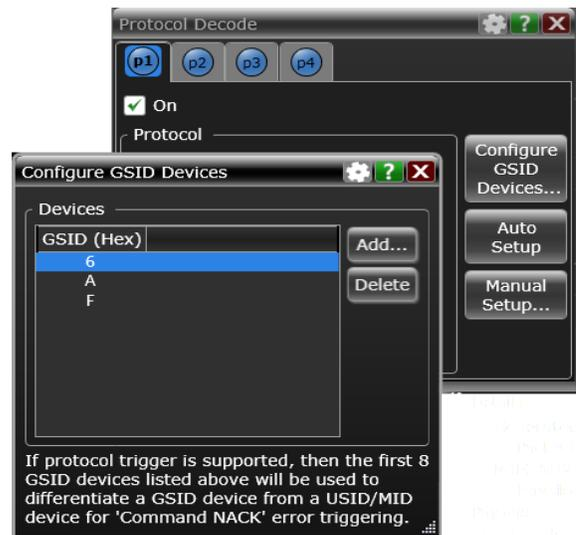
Figure 4. Because of differences between USID and GSID, D9010MPLP allows for the configuring of GSID of up to 8 sets allowing the systems operator to identify proper behavior depending on GSID address.
