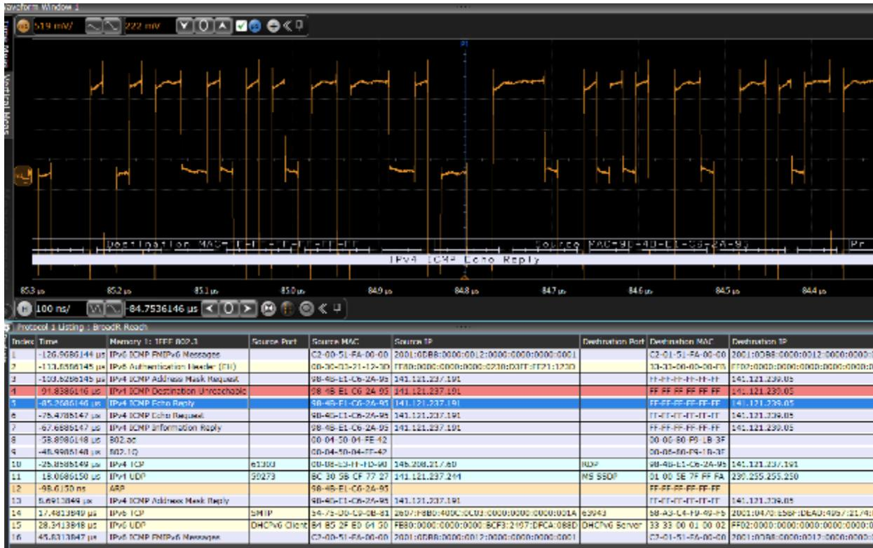
Display as many protocol packets as you want to see. The protocol viewer shows index number, time stamp, and data content for each serial packet. Listing content can be saved to a .csv or .txt file for off-line analysis or documentation. Use search capability to quickly navigate through an acquisition.
