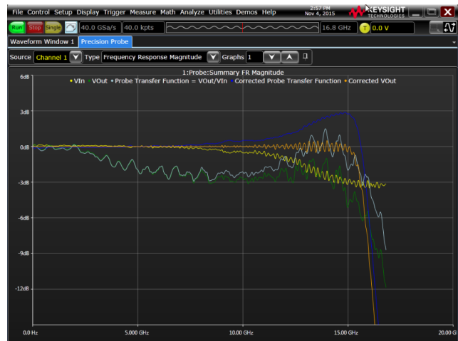
Figure 4. This chart shows the probe/cable's frequency response magnitude and the corrected response.
