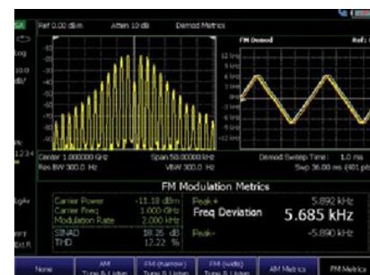
Characterize AM/FM signals using AM/FM demodulation
