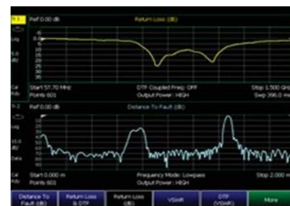
View return loss and DTF simultaneously
