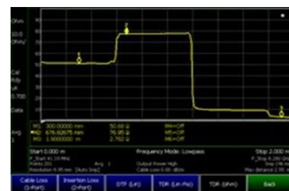
Gain insight into faults with TDR measurements
