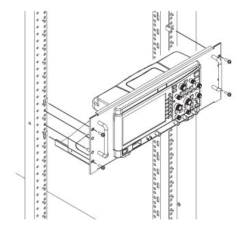
**3** Fasten the support shelf to the rack cabinet using four 10-32 dress screws. This completes the installation.
