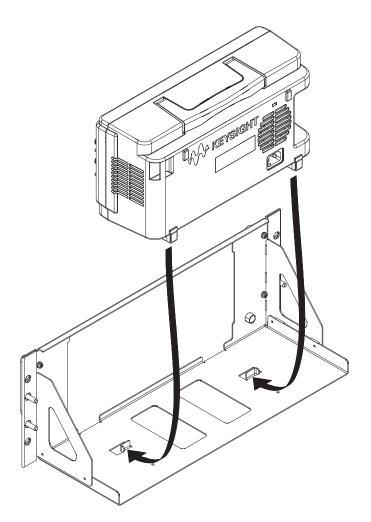
2 Push the oscilloscope fully forward on the support shelf assembly.
