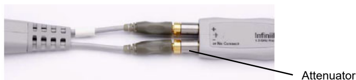
Figure 3 Attenuators Between a Probe Amplifier and a Probe Head
