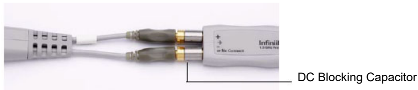
Figure 77 Placement of DC Blocking Capacitor Between a Probe Amplifier and a Probe Head
