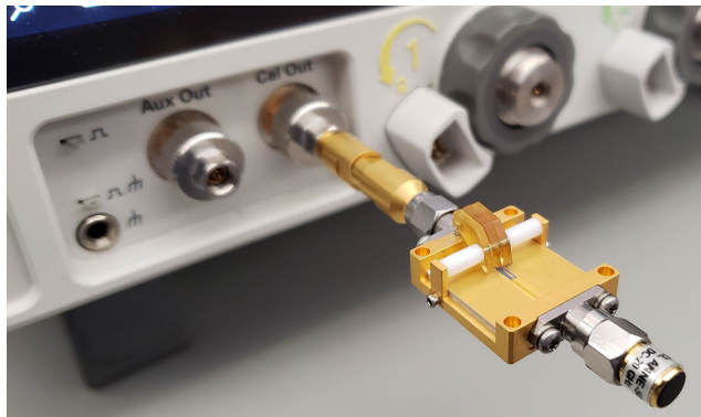
Figure 74 MX0104A deskew fixture connected to oscilloscope's Cal Out connector
