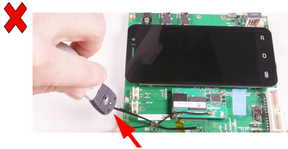
Figure 23 Example of incorrect movement of MX0100A probe head
