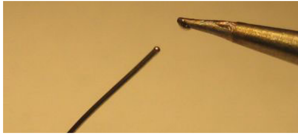
Figure 57 Small Amount of Solder Added to Soldering Iron Tip
