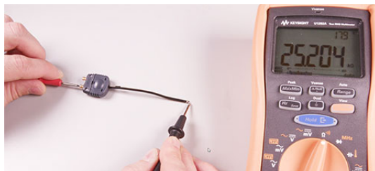
Figure 24 Resistance measurement for an undamaged MX0100A probe head
