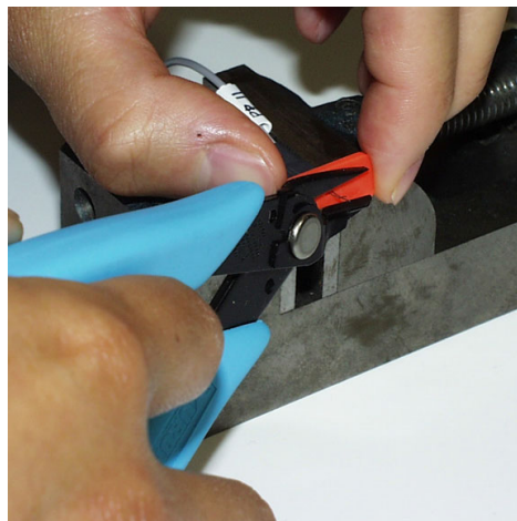
Figure 32 Cutting Wires Flush with Gauge
