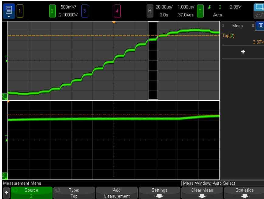
Figure 47 Isolating area for Top measurement
