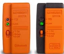
Keysight U1177A Infrared (IR)-to- Bluetooth adapter
