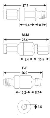
Dimensions in millimeters Net Weight: 14 Grams each
